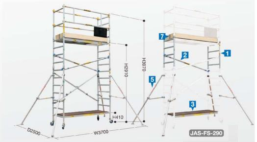
Please let the scaffold vertical stand up and open it to opposite direction. Make sure the folding joints are all in straight direction. Please make sure four of wheels are all locked.
